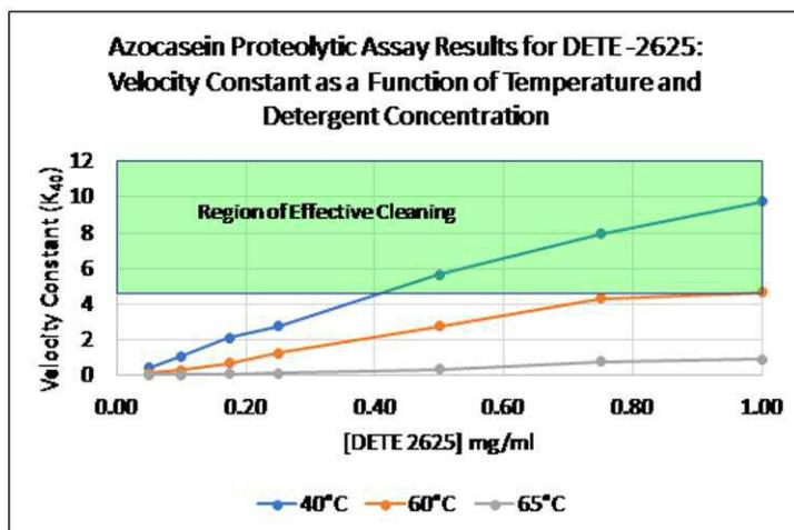
usage at 65°C would have been apparently justifiable. The cleaning indicator correctly indicated that use of this detergent at 65°C was not appropriate for all washer-disinfector designs.
