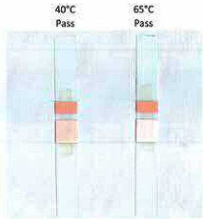
above. Recall that in the Miele washer-disinfector, the enzymatic cleaning actually takes place while the detergent heats from room temperature on its way to 65°C; this explains this apparent contradiction.
